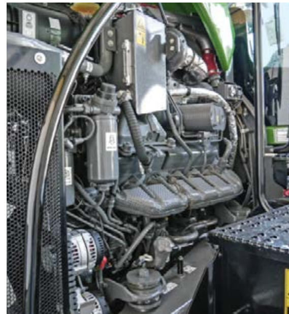
■ The 12-cylinder AGCO Power engine convinces you with its smooth running and good maintenance access.
