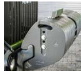
■ Marginal 990 kg weight can be mounted on the front frame.
