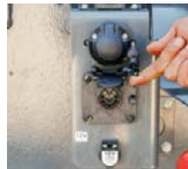
□ A 12 V connection is available at the rear for external consumers. The ISOBUS connection establishes a connection with attachments.
