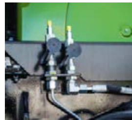
■ In order to tension the rolling tracks, the pressure connections are easily accessible.
