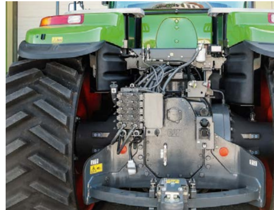
The drawbar, steered hydraulically through 28° on each side, controls the attachments to perfection.
