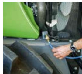
□ A compressed air connection is located at the front to clean the radiator.
