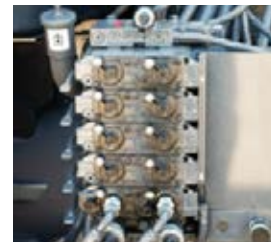
■ Six hydraulic valves, a leak-oil line connection and PowerBeyond are located at the rear.
