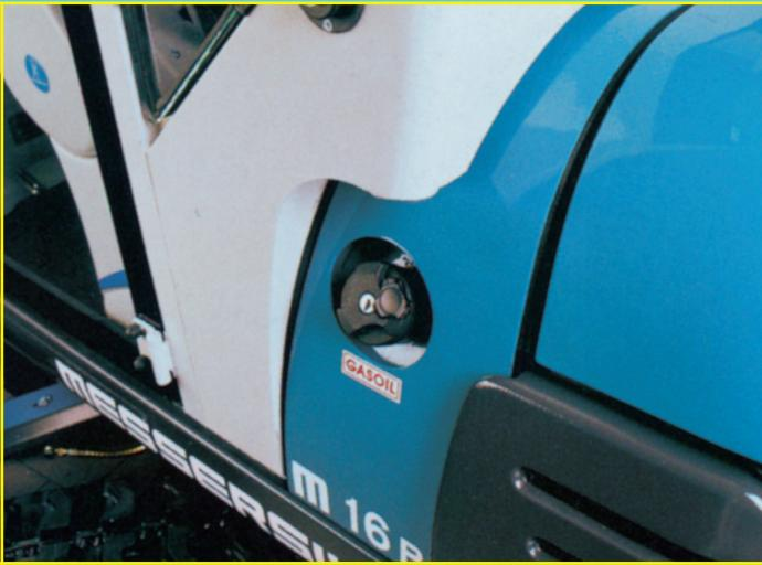
Refuelling access is external to the engine compartment
