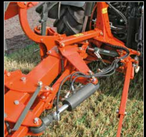
Variomat® for RM2000V-RM2005V Parallel linkage with memory cylinder and hydraulic front furrow adjustment
